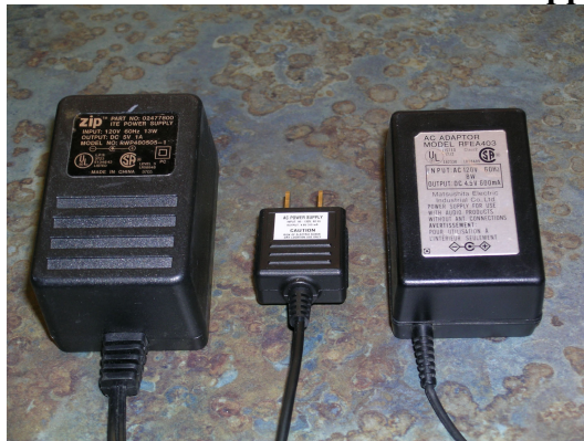
Figure 3. Comparing the Size of an Efficient (Middle) and Two Inefficient External Power Supplies
