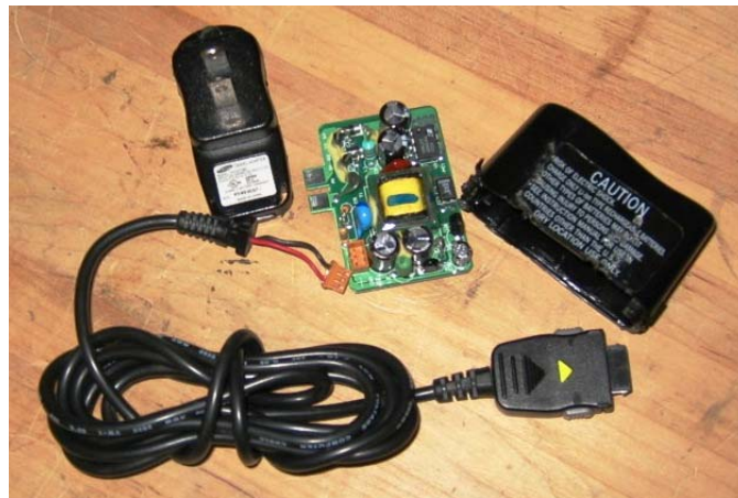
Figure 9. A switch mode charger designed to charge a cell phone battery.
