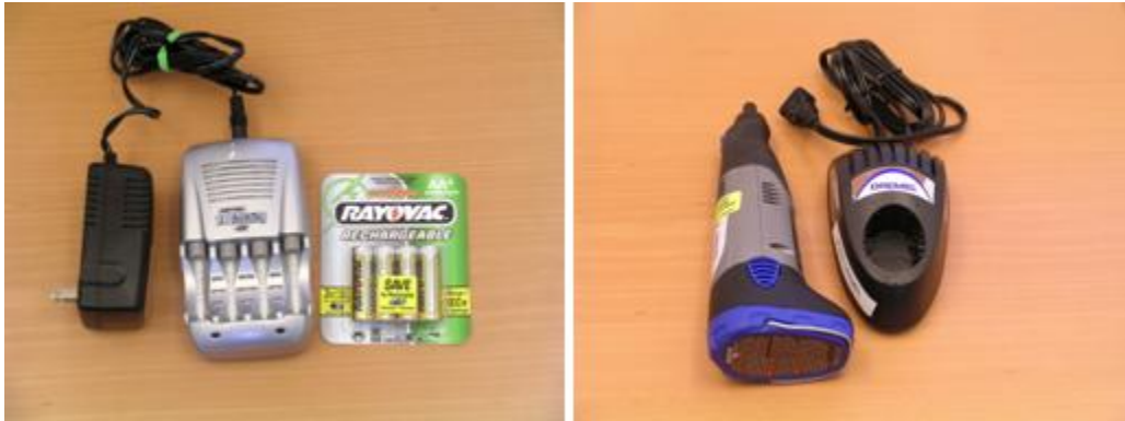
Figure 3. A multi-piece battery charger for AA batteries (left) and a single-piece battery charger for a power tool (right). Note that the multi-piece charger connects to ac with an external power supply.
